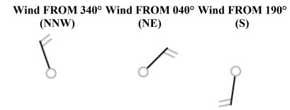
The wind direction is indicated by the long shaft. The shaft will point to the direction FROM which the wind is blowing. The direction is based upon a 36-point compass.
